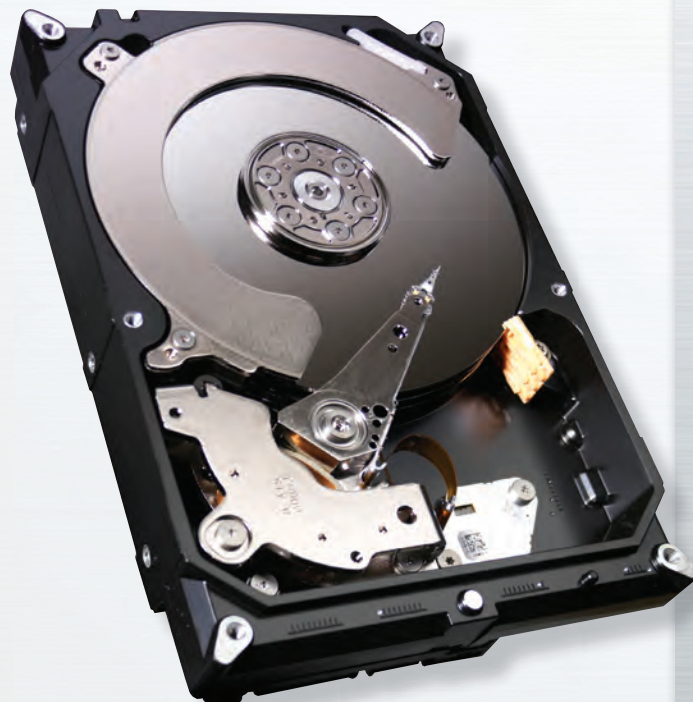
A hard drive uses magnets (lower left) to move the read/write heads (the pointy things), which are both above and below the data platters.
